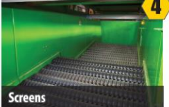
Screens Separates material by size at various points in the system
