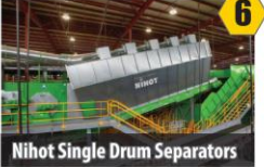
Nihot Single Drum Separators Separates heavier material from lighter, high-value recyclables
