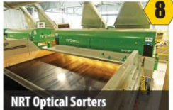
NRT Optical Sorters Uses near-infrared technology to remove film and plastics
