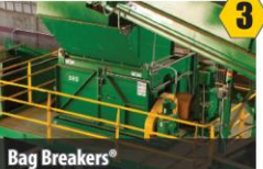
Bag Breakers® Open bags without damaging material
