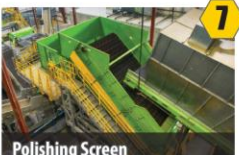
Polishing Screen Separates mixed fiber from containers & removes any remaining fines
