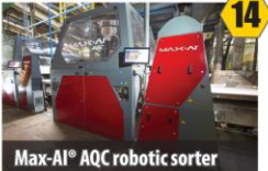
Max-AI® AQC robotic sorter Robotic sorter removes containers from 2-6" heavies line
