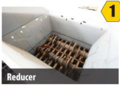
Reducer Sizes material and provides a metered & consistent infeed
