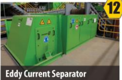
Eddy Current Separator Captures aluminum cans
