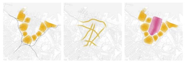
Figure 12: Diagrams showing traffic access points and low-traffic zones surrounding the city center (left); priority transit routes on arterial roadways connecting between regional routes (middle), and the pedestrian-priority "zero emissions area" planned for the core of the city center surrounded by low-traffic zones(left) Source: Auckland Council (44)
