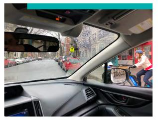
At a protected intersection, the bike lane is set back from the motor vehicle through/turn lane, so the bike rider is visible as the driver turns.
