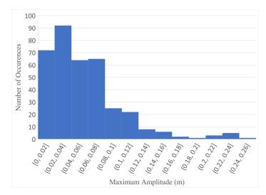
**Figure 5.** Histogram of the maximum wave amplitude at site RM 42-1.
