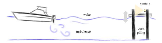
Figure 1. Recreational boat wake and dock interaction, with the generalized experimental setup.
