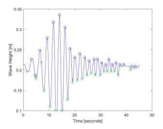
**Figure 4.** Example of a wave height calculation from a video on site RM 42-1 recorded in late May 2019. Circles indicate the maximum and minimum height of the wave calculated by the algorithm.
