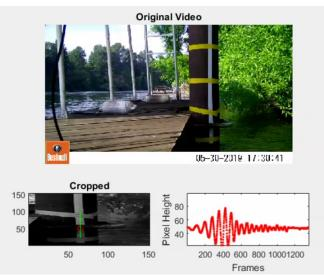
**Figure 3.** The Matlab screen used by the research team for monitoring the calculations. The upper image is the original video, the lower left shows the green vertical line of pixels where the tracking is occurring. The lower right shows the pixel height measurement over each frame of the video.
