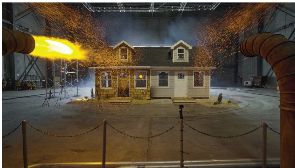
Figure 3. The Insurance Institute for Business and Home Safety crash tests buildings to determine vulnerabilities to flood, wind, fire and natural forces. The research shows the mechanisms by which a home ignites from burning embers in extreme fire weather and how to significantly reduce the chance a home will ignite. Photo credit: ElementalFilm.com.
