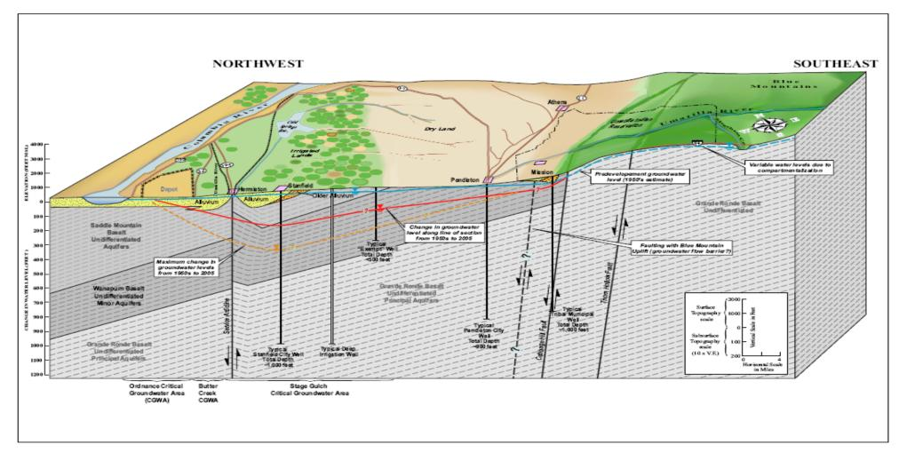
Figure 26: Graphic representation of the Umatilla Groundwater Structural Basin (OSU/IWW). Note that the current picture reflects that the basalt groundwater system is interconnected like a bath tub. Further research is necessary to accurately depict the compartmentalization and interconnectivity of the basalt groundwater resource.
