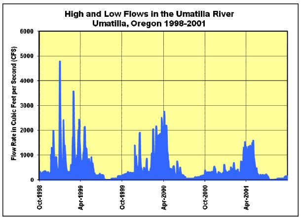
Figure 7 and 8 - Daily discharge in the Umatilla River near the confluence with Columbia River at river mile 2.1 for the water years 1999 through 2001 and monthly discharges at UMAO from 1930 to 1997. Note that the hydrologic pattern is highly variable showing a strong correlation to winter snow pack and run-off (Ely, 2005)
