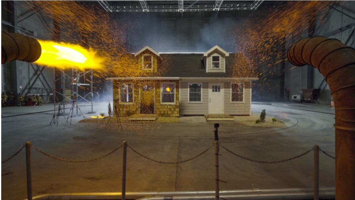
Exhibit 1 - IBHS Facility, South Carolina - The wildfire-prepared side did not ignite and burn.
