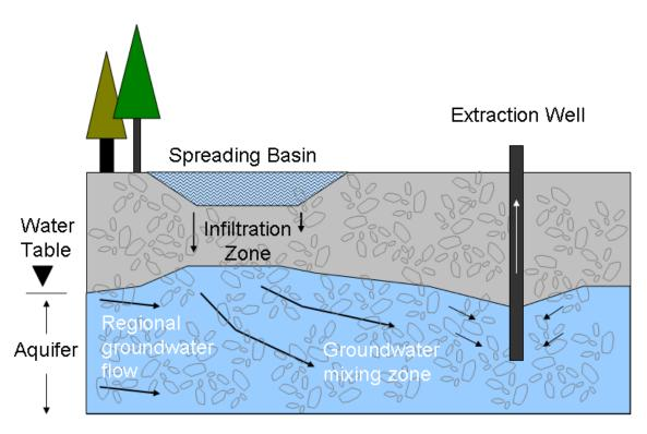
Figure 3. In a typical spreading basin project, water infiltrates through shallow basins or canals. Withdrawal occurs down gradient through a well or the water discharges to the surface and augments stream flow.
