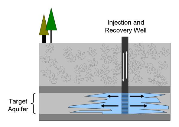
Figure 2. In a municipal injection and recovery system, surface water is treated to drinking water quality, stored underground, and later withdrawn and distributed to water customers.
