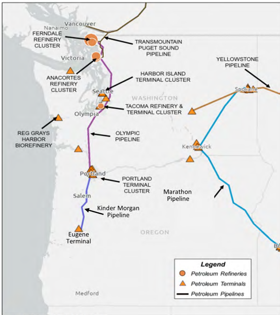
Figure 23: Map of Pacific Northwest Critical Petroleum Infrastructure 26
