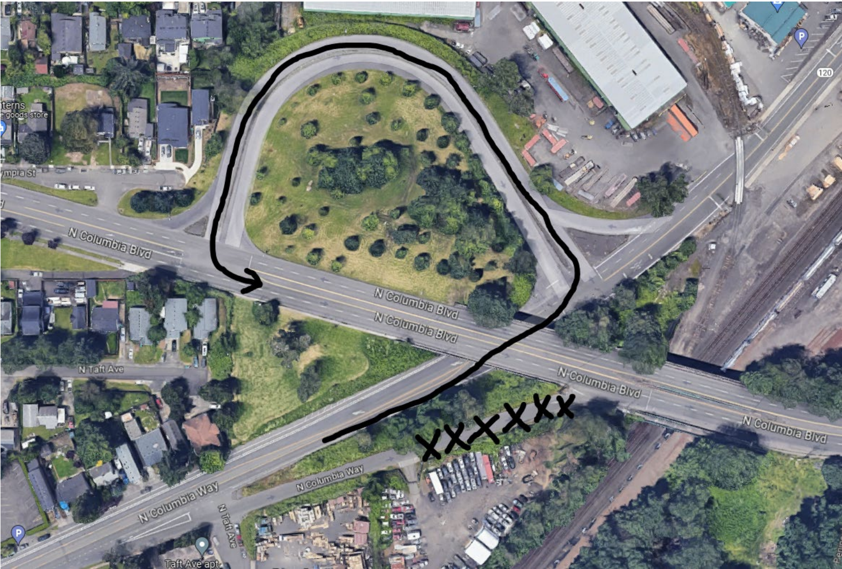
Traffic circulation change needed due to higher grade of bridges and roadway
