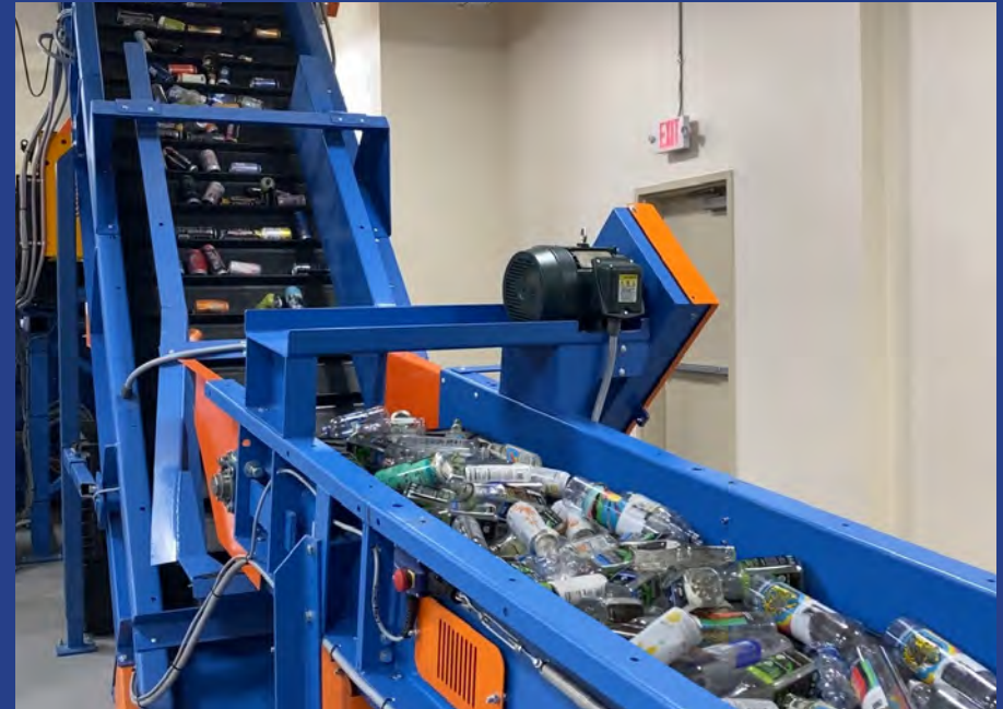
Glass, plastic and aluminum beverage containers enter an OBRC Material Separation Unit.
