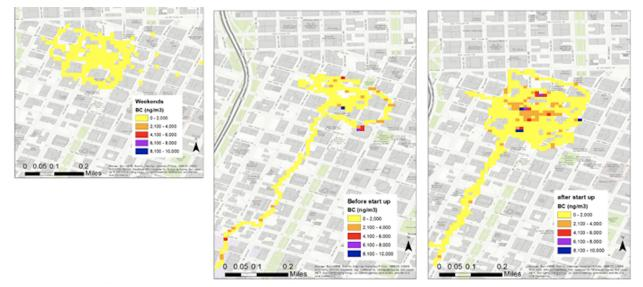
**Figure 1**. Measurements of black carbon around a major downtown Portland construction site in Fall 2019, (left) on the weekend, (middle) before construction operations start on weekday mornings, (right) during construction operations. Figure credit: Kirsten Sarle, Portland State University.
