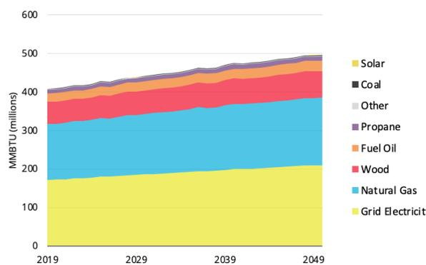
Figure 13. Energy consumption by fuel type in the BAU scenario, buildings sector
