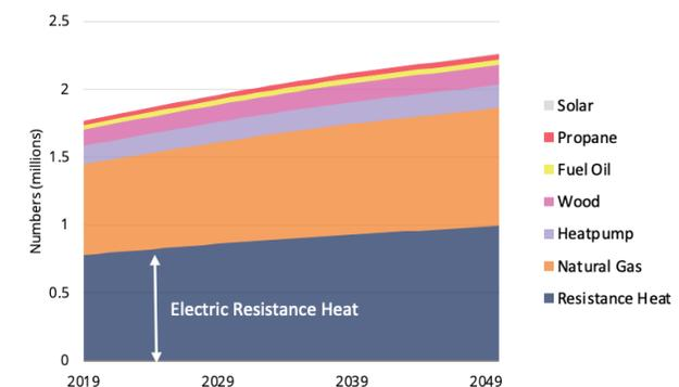
Figure 14. Number of heating systems by type in the BAU scenario, buildings sector
