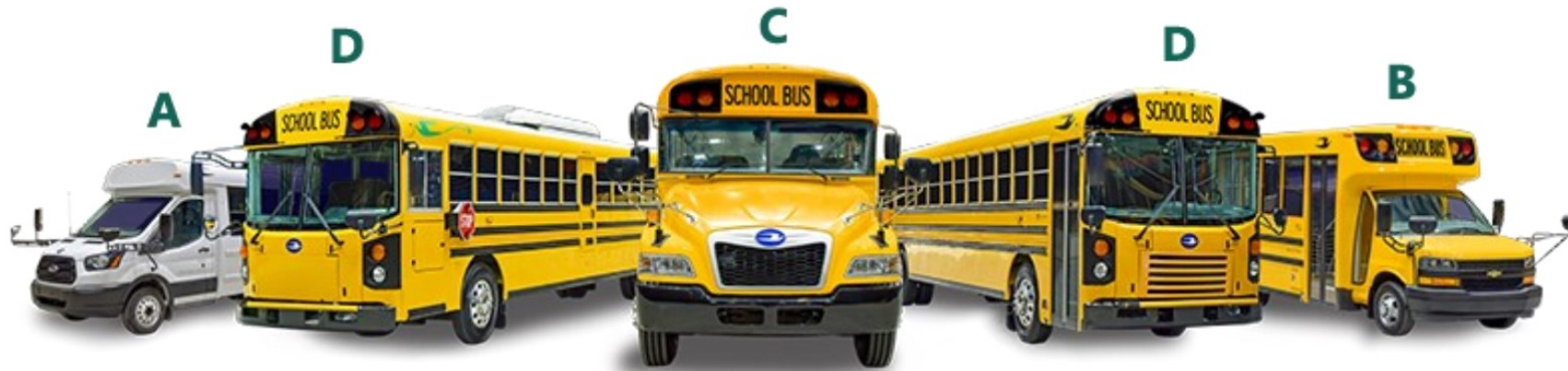
Buses shown are examples of types A, B, C, and D. Photo source: blue-bird.com
