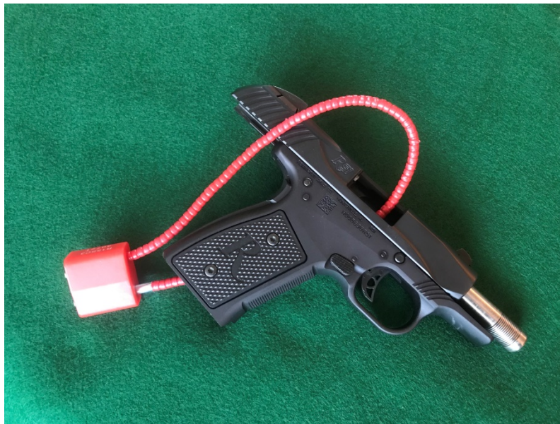
Cable lock on 9mm handgun. Using a cable lock this way, you know that the handgun is unloaded and can't be fired.
