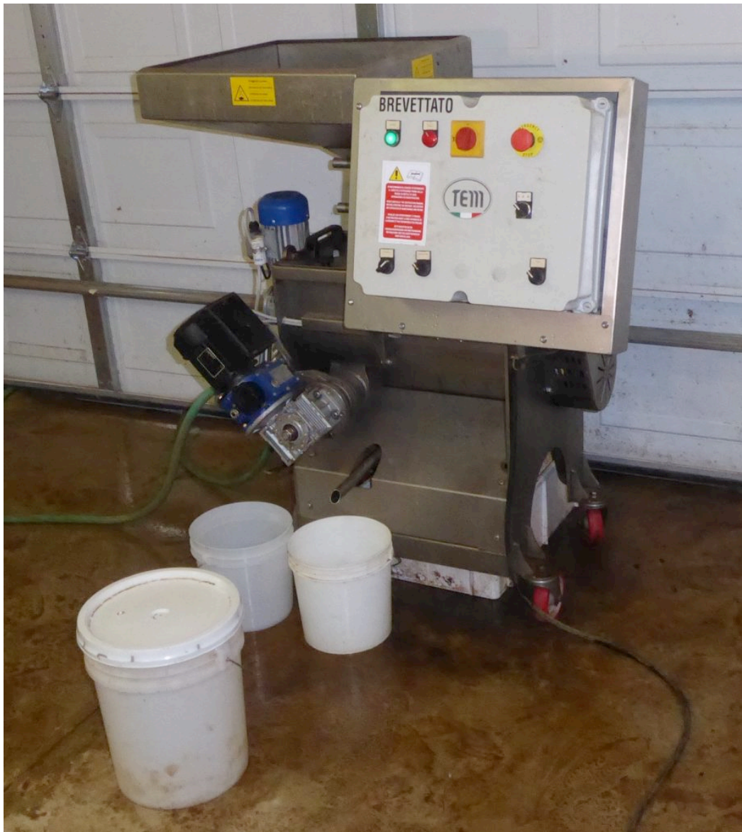
Our small, fully modern 2 phase centrifuge based olive mill. Two gallon and five gallon buckets shown for scale.
