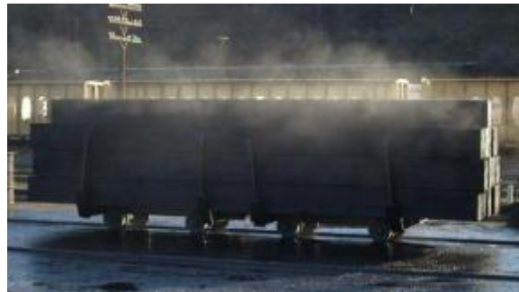
Wooden rail ties at the AmeriTies plant in The Dalles are treated with creosote to protect against the elements.
