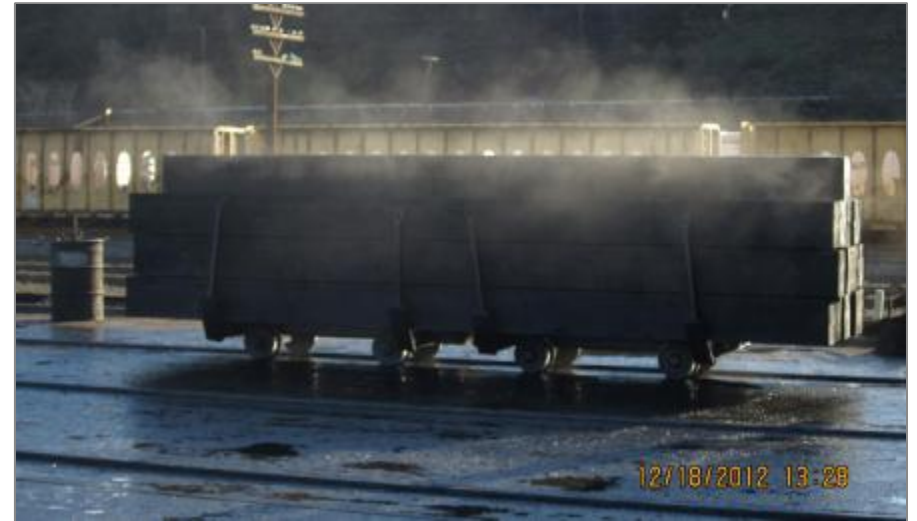
A Department of Environmental Quality photo of rail ties releasing vapors at the plant in The Dalles.
