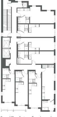
Carmel Place features five micro-unit floor plans that vary in size and configuration. Most floors of the nine-story building include all five arrangements (shown in the plan above).
