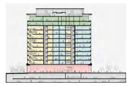
A section view shows an internal staircase (left side) that connects the floors within each of the building's three-story "neighborhoods." Rendering ©Perkins Eastman, courtesy WeLive
