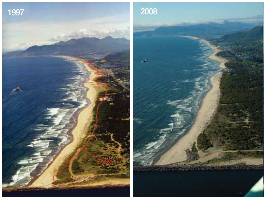
North Oregon coast showing 1997 high-water line (red line) moving inland by 2008 (Allan, 2009). Photos by Don Best.
