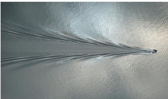
Figure 2. Pattern of vessel-generated waves in deep water. Diagram from Sorenson 1973.
