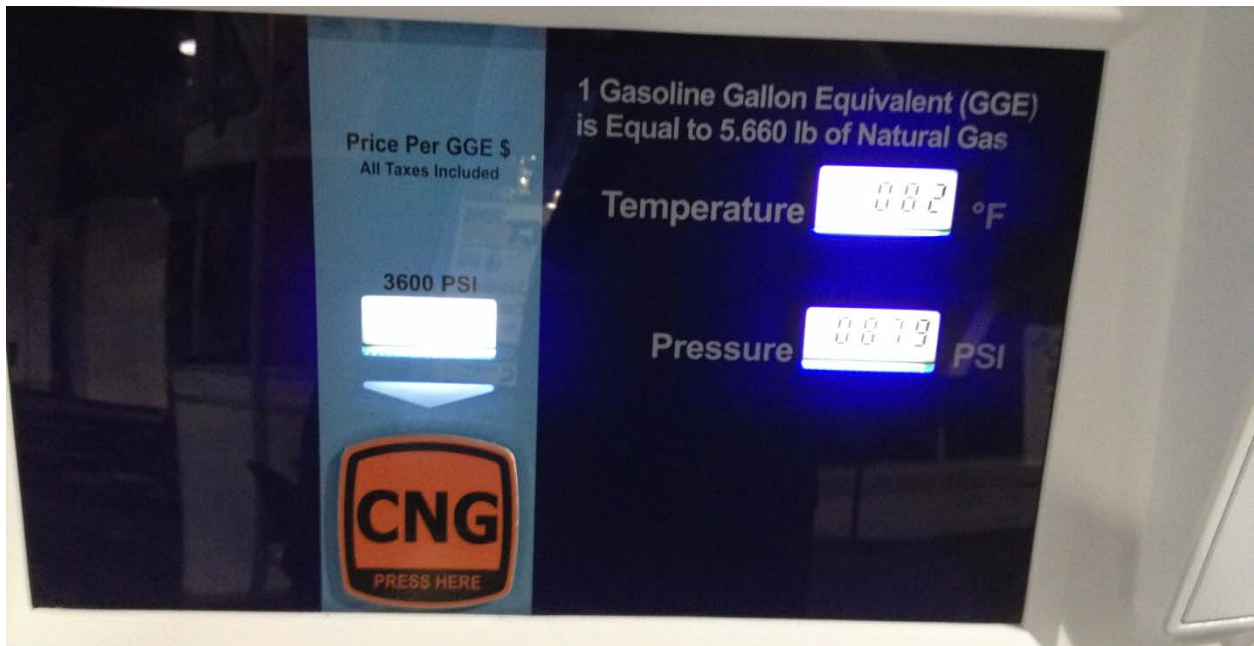
Figure 5. An example of the compressed natural gas conversion factor for gallon equivalent at the pump.
