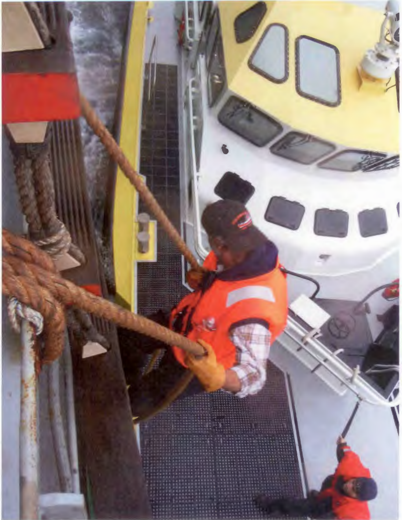
Descending to the pilot boat from the ladder using manropes.
