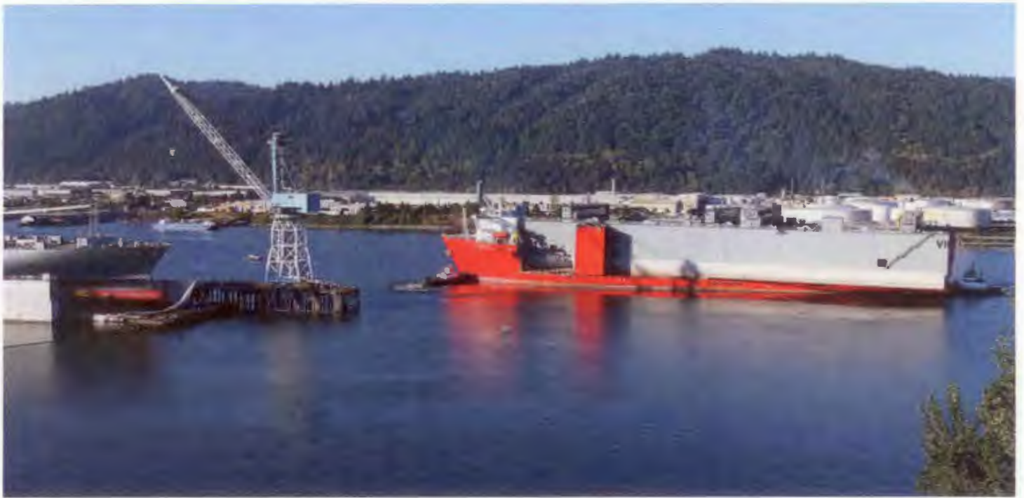
More images of the dry dock Vigorous on its transit to Swan Island. It was transported by the world's largest heavy-lift ship. Arriving in three parts, it was later assembled into a single 960-foot long unit.
