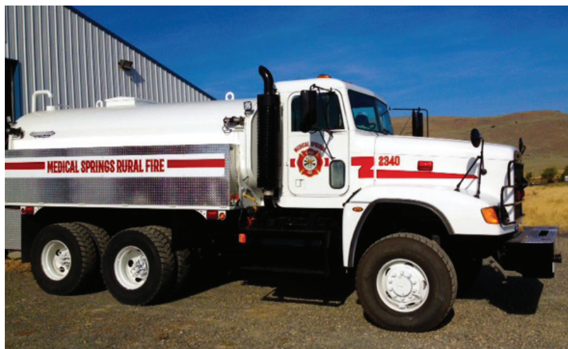
The Medical Springs RFPD's new water tender was constructed from a donated chassis and a new water tank purchased with a USDA grant.
