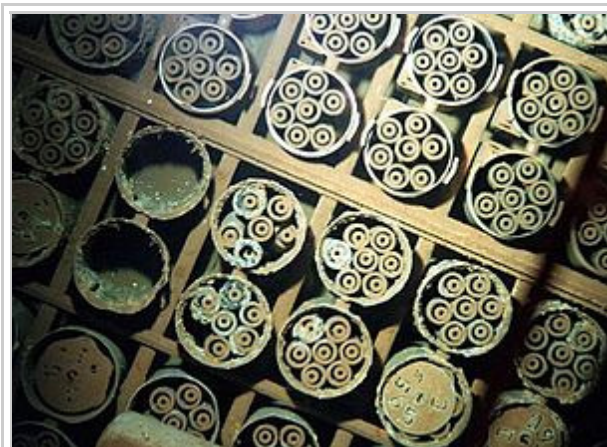
Spent nuclear fuel stored underwater and uncapped at the Hanford site in Washington, USA.
