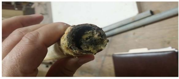
Picture of galvanized, deteriorated, and corroded pipe from Douglas County courthouse
