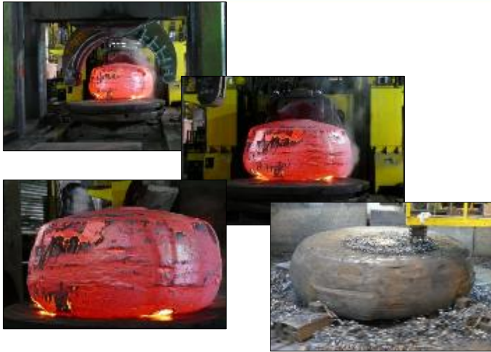
NuScale RPV Head Ingot Being Forged
