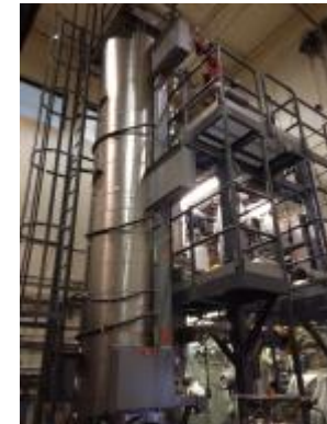
One-third scale NIST-1 Test Facility
