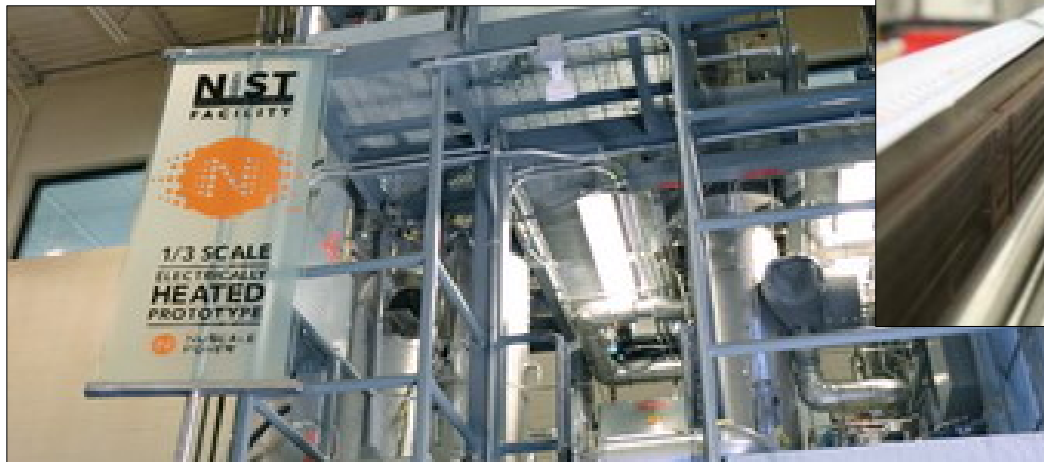
NuScale Integral System Test Facility (Oregon State University)
