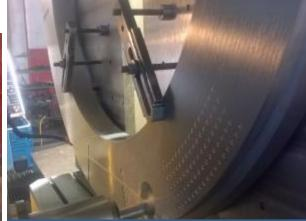
Machining of Tube Sheet
