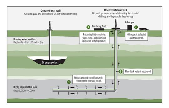
Figure 1: Basic comparison of a conventional vertical hydraulically fractured well versus an unconventional horizontal well. An unconventional directional well would not begin on a vertical decent, it would descend direction, and would most likely become horizontal, once located in impermeable rock formations (Office of the Auditor General of Canada 2012).
