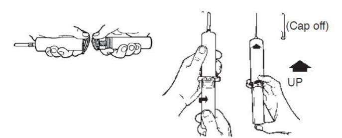
Align vial such that the injector needle is centered on the stopper.
