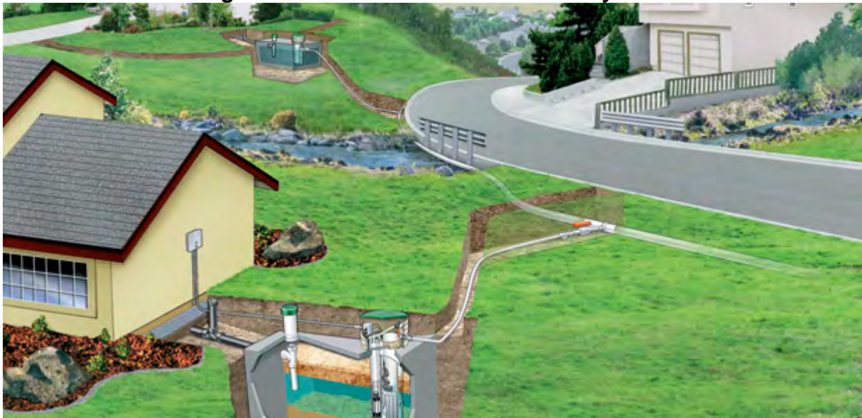
Figure 5.1 Effluent Sewer Collection System
