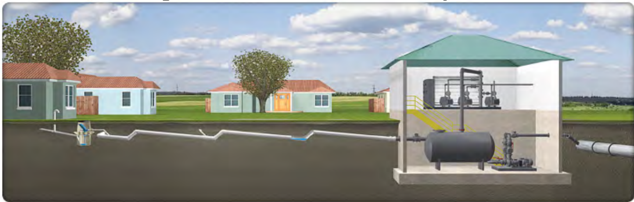
Figure 5.2 Vacuum Sewer Collection System
