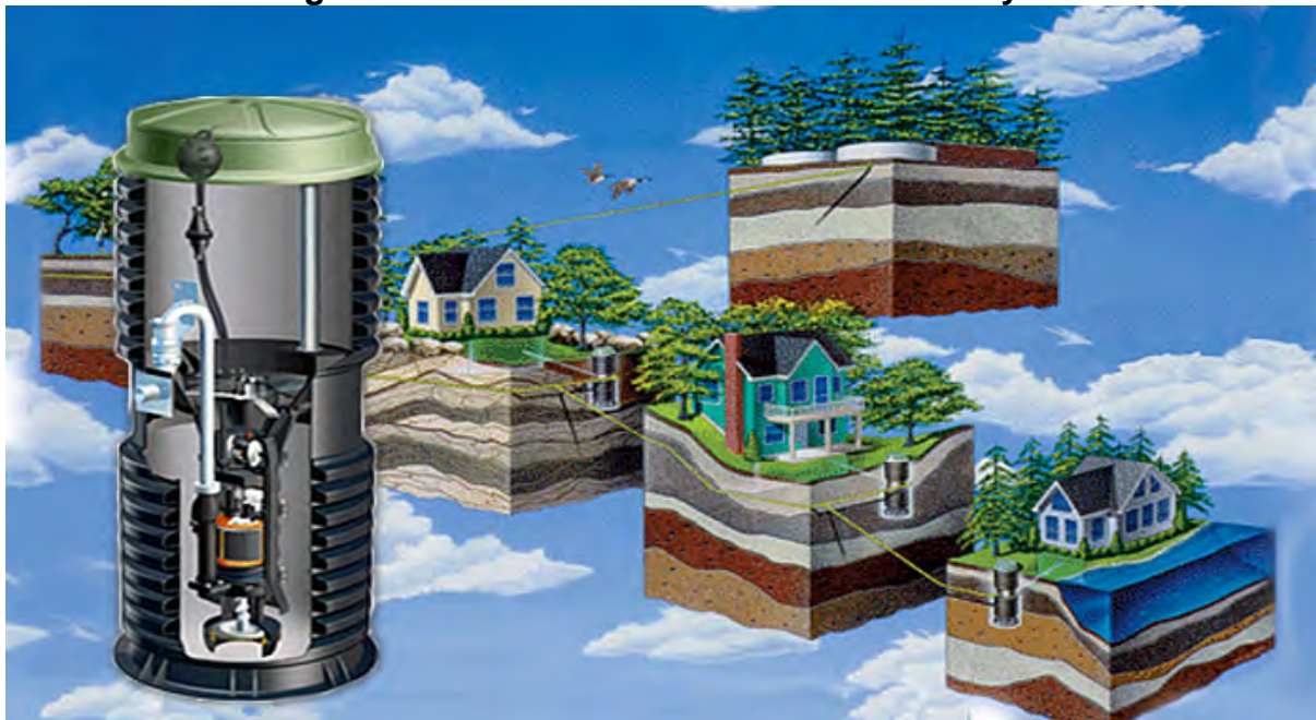
Figure 5.3 Low Pressure Sewer Collection System
