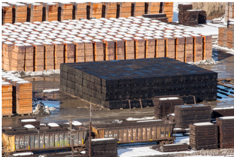
Behind railroad cars, dark treated ties are stacked. Light-colored untreated ties await treatment behind them.
