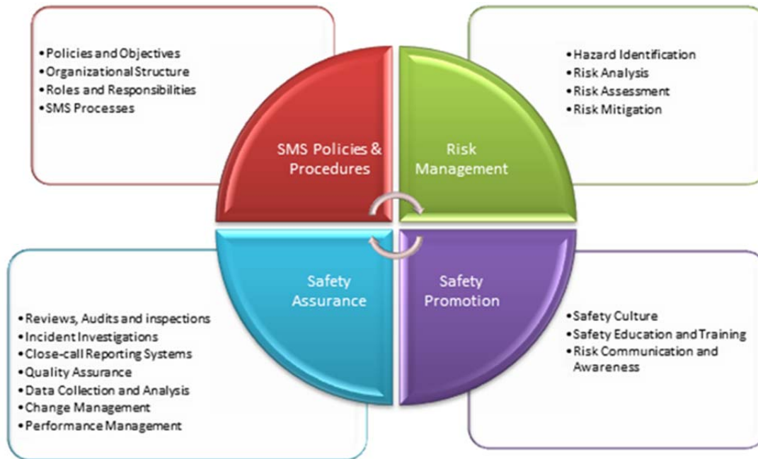
Figure 1. The Four Pillars of Safety Management Systems (SMS). (Source: TRACS 12-02 Report , p. 12)
