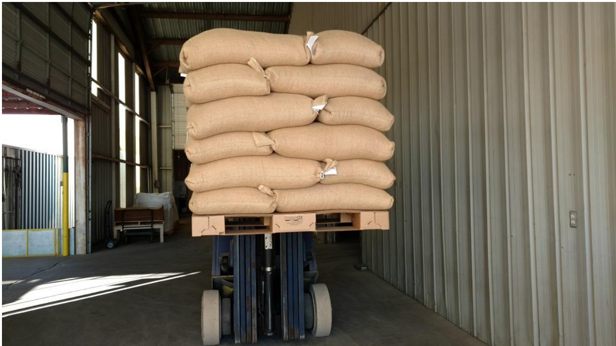
Lightweight corrugated cardboard pallets are as effective as other pallets. Photo Credit: Change the Pallet
