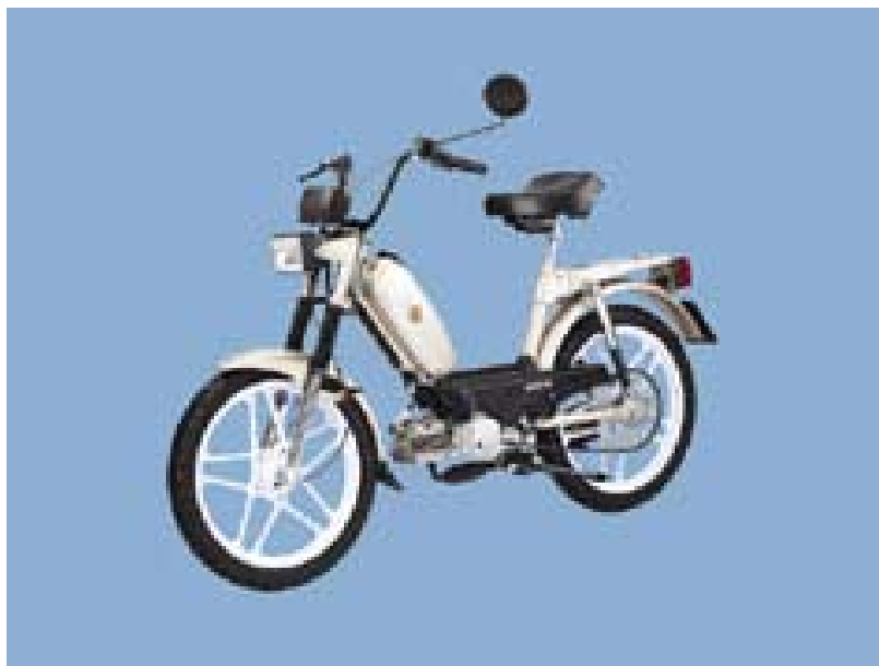
Figure 2.7: Step-through style PTW
