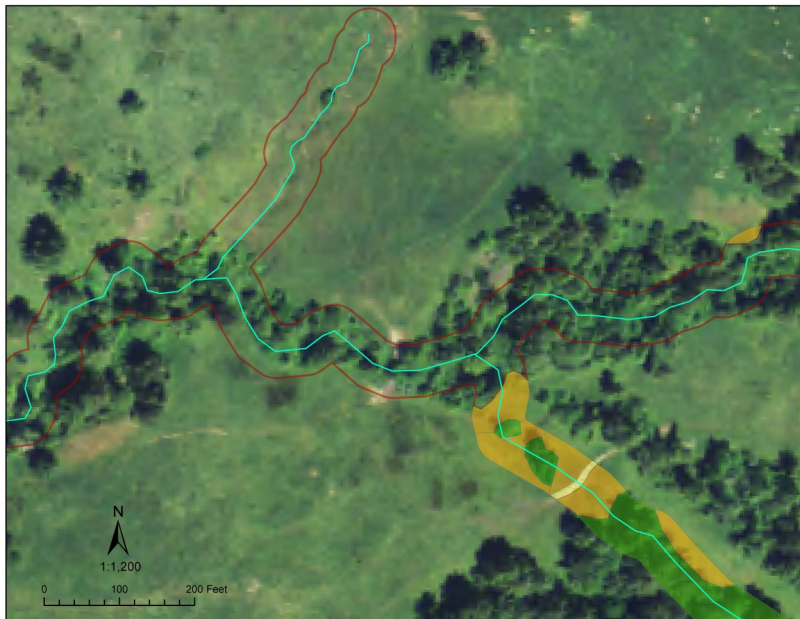
2012 Aerial photo with SVA assessment polygon (red), stream centerline (teal) and the SVA mapping categories.
