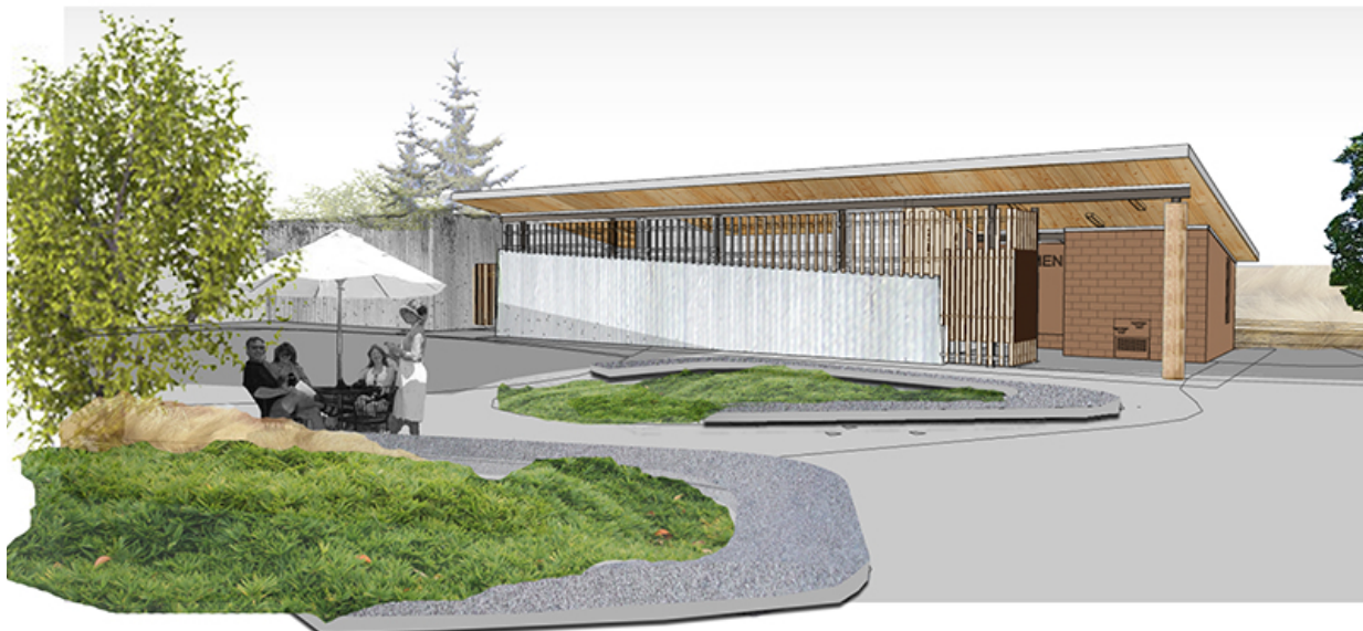
Photo Credit: EMILY DAWSON OF SRG PARTNERSHIP IN PORTLAND - Architect's rendering of a new visitor's center at the Oregon Zoo. The large slab on the roof is cross-laminated timber.
