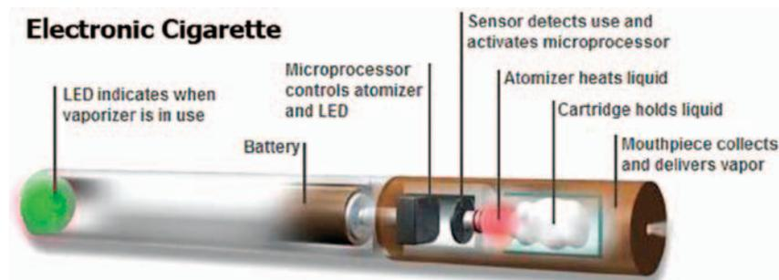
Figure 1. Image of cross section of e-cigarette components.
