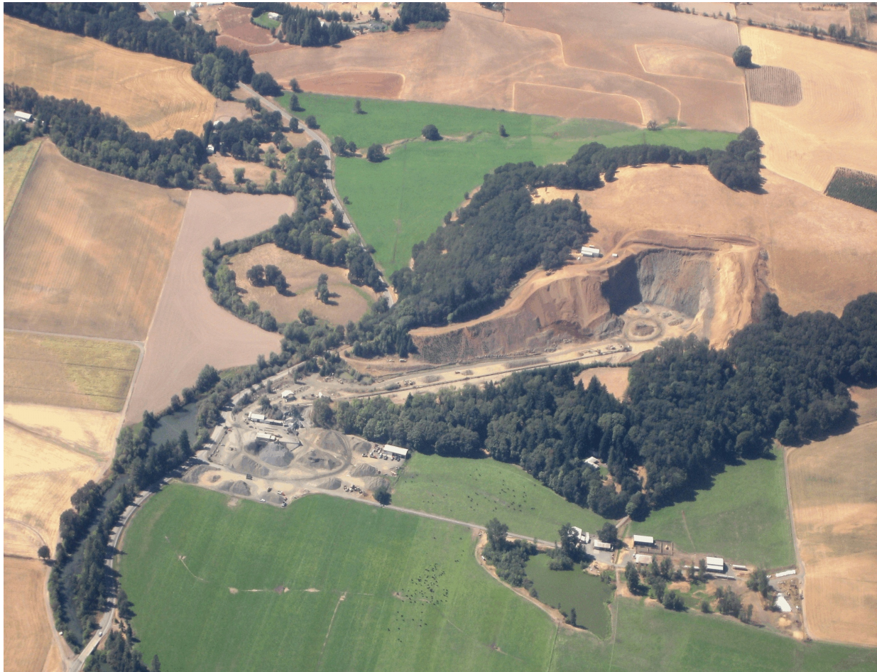
Figure 3. Basalt quarry in the southern Willamette Valley. The hill is underlain by basalt that is mined and crushed on site. Soils overlying such uplands within and along the Willamette Valley are largely poor for farming, Class 5 and higher, with some areas of Classes 3 and 4. Basalt deposits such as the one pictured here are typically much more than 100 ft thick, providing a large amount of rock from a small area of disturbed land.
