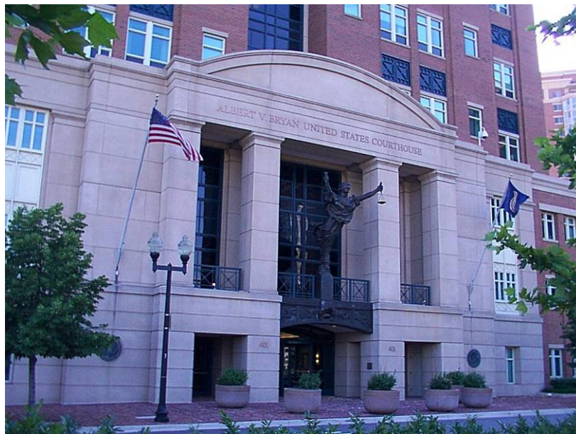
Figure: Courthouse without plinth for easier access.
