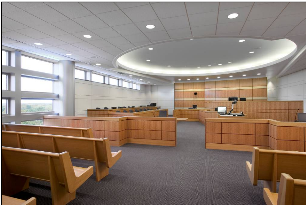
Figure: Main aisle in courtroom of adequate width and rail without gate
