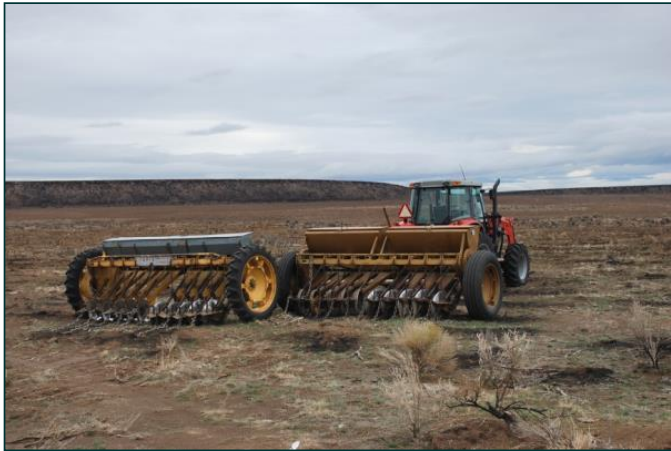
Rangeland drill used to reseed burned areas
